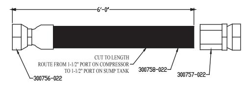
NOTE: THREE HOSE ASSEMBLIES ARE REQUIRED CUT HOSE SO ONE ASSIMBLY HAS ONE 90<sup>®</sup> CRIMP FITTING AND ONE REUSABLE FITTING, THE OTHER TWO ASSEMBLIES WILL HAVE TWO REUSABLE FITTING ON EACH END
