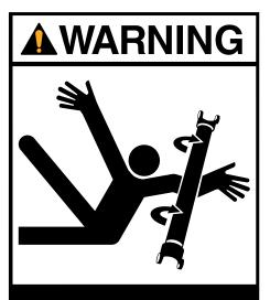
Driveshaft in rotation. Switch off engine and disconnect battery or electrical supply before attempting to work or perform maintenance on the compressor package.
