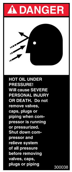
Hot Oil Under Pressure: Placed on body near oil sump filler cap.
